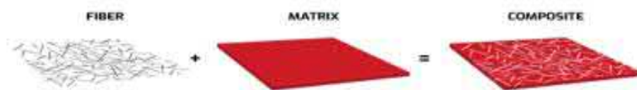
Figure 9: Schematic composition of composite 11
