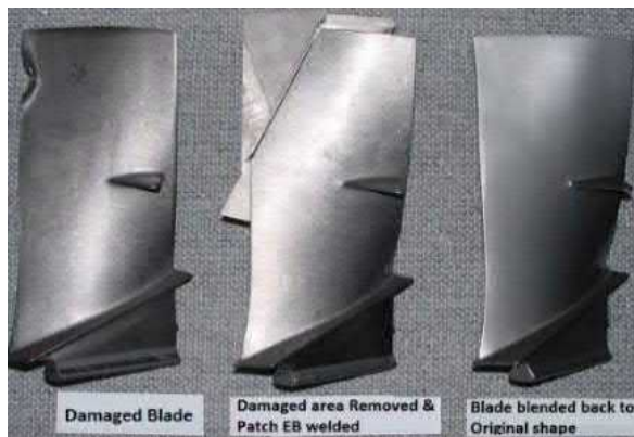
Figure 5: Fan Blade Repair with EBW
