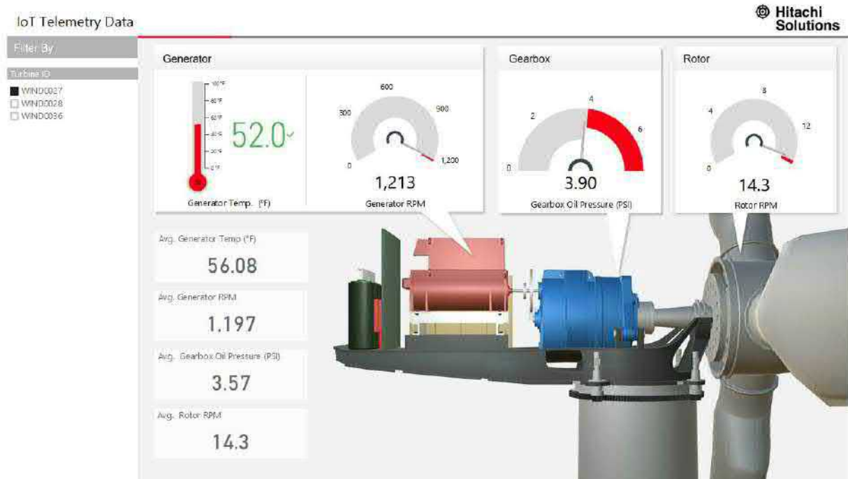
Fig 6: Data collection for monitoring a turbine (Thanks to Hitachi solutions)
