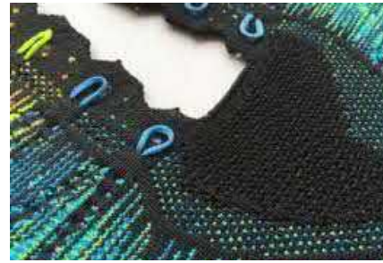
Figure 12: Illustrative figure of circular knitted upper
