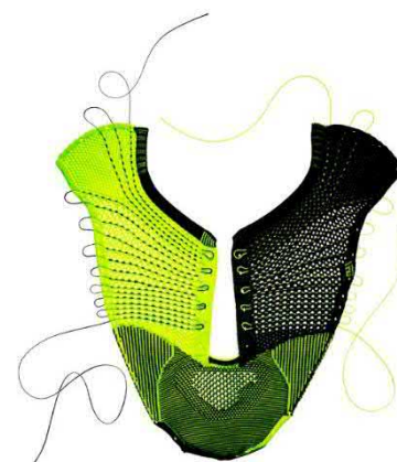
Figure 11: Illustrative figure of 2D knitted upper
