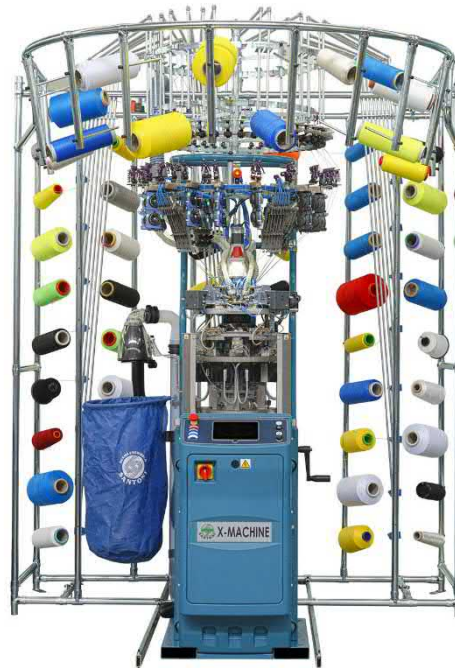
Figure 10: Illustrative figure of 3D upper knitting machine
