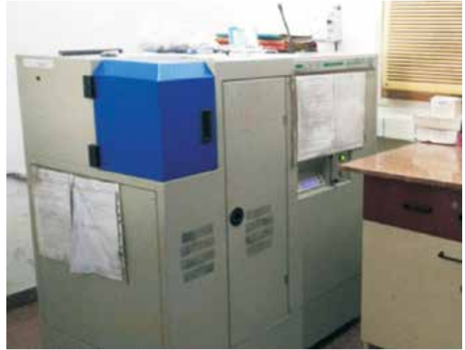
Spectro Meter-For Chemical Analysis of Metals
