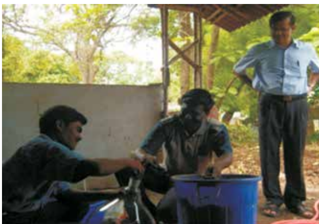
Filling of cleaned hair in the reactor for hydrolysis
