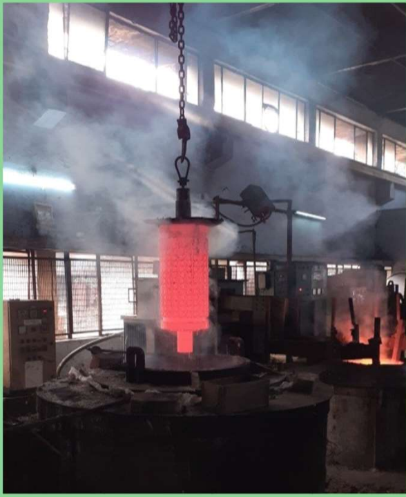
Heat treatment of critical peripheral design roller die for producing Papdum (Food item) by using salt bath HT technology
